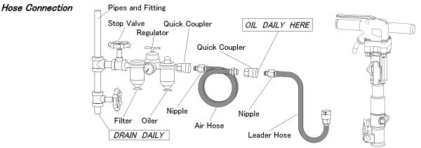
Whether there is any dust, or damage to the air connection portion. Whether the air hose is tight enough.
